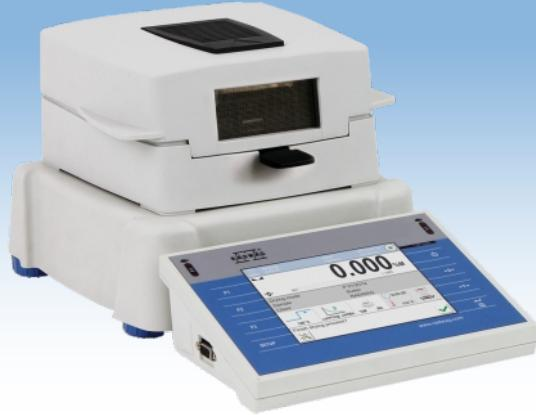
Moisture analyzer is a laboratory measuring instrument intended to determine relative moisture content in samples of different substances. **MA 3Y** features 5,7" LCD colour touch panel which provides new possibilities of instrument's operation and presenting measurement results. It features extended databases containing programmable drying modes related to the database of samples. MA 3Y series enables printing and exporting charts presented on its display to a BMP file.
